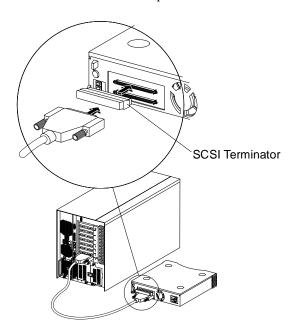
Figure 1-10. Connecting External SCSI Devices
